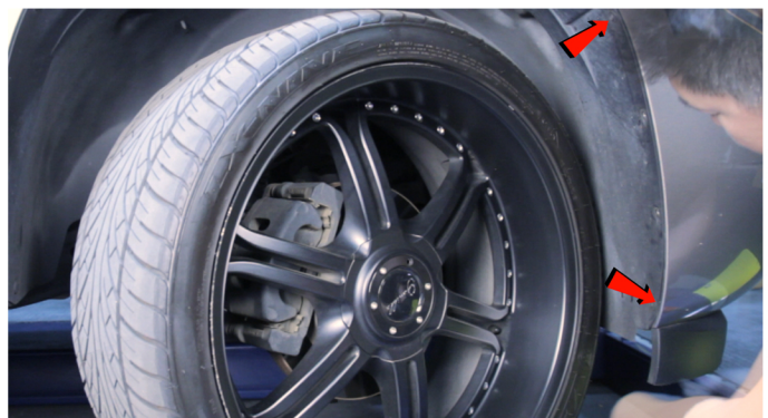
4) Remove the [2x] 7mm bolts securing the fender liner.
