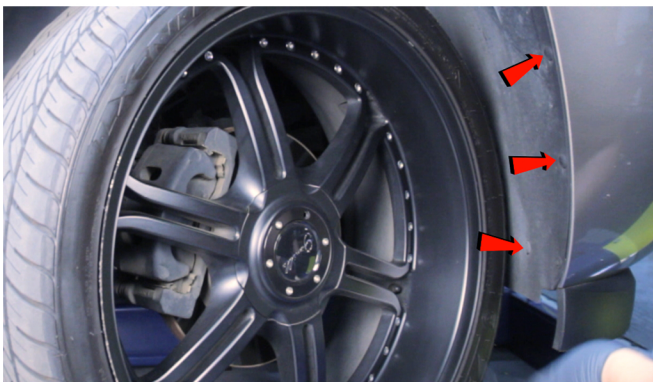
3) Remove the [3x] plastic retainers securing the fender liner using a panel popper tool.
