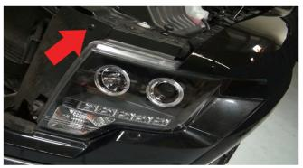
1) Open your hood and locate the plastic Phillips screw that is holding the headlight shroud. Once the plastic Phillips screw has been removed with a Phillips screw driver, fold the shroud back to access the (3) 10mm bolts.
