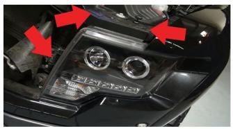
2) Once the shroud has been folded to the side, you will be able to access the (1) 10mm bolt behind it. Remove (2) 10mm nuts, shown on top. Unscrew these bolts and set aside for later use, as you will reuse these bolts to secure your new Spyder light.
