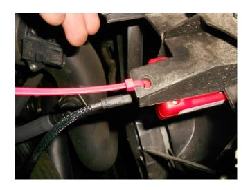
6. The module is to be secured using the included zip-tie. Please note -- DO NOT route the zip-tie over the harness at the module, as this could stress the internal circuit board and damage the module! Only insert a zip-tie thru the slots on the module as shown
