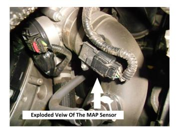
4. Carefully unplug the sensor. There is a locking tab located at the top of the sensor, squeeze the tab and pull the plug to remove.
