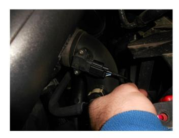
8. Connect the male connector on the Delta Boost module to the factory female connector on the wiring harness.
