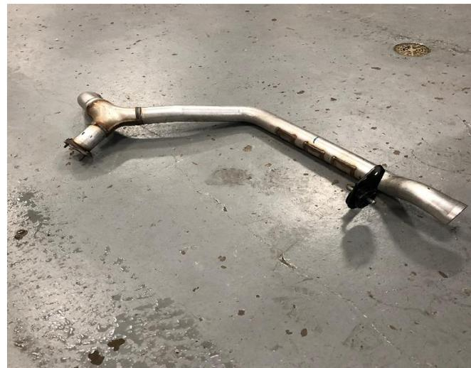
**12.** Carefully remove the passenger side tail pipe section.
