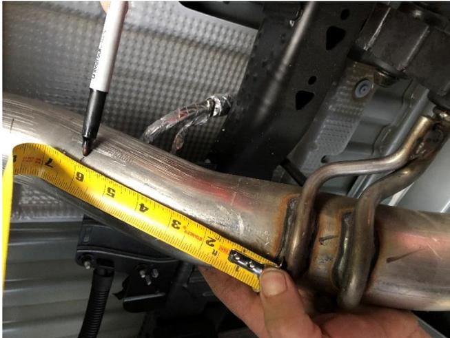
1. Scribe a line 6" from the hanger next to the muffler closest to the rear of the vehicle.
