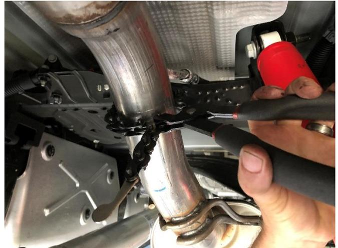
2. Place a chain style cutter around the exhaust pipe at the scribe line location and cut the exhaust pipe.
