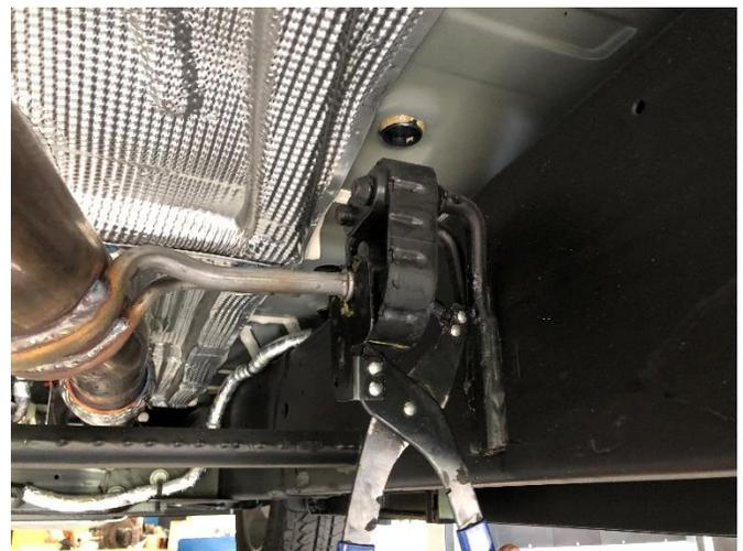
4. Remove the grommet from the Headpipe hangers at in the front of the muffler behind the flex pipe, using grommet pullers or similar device.
