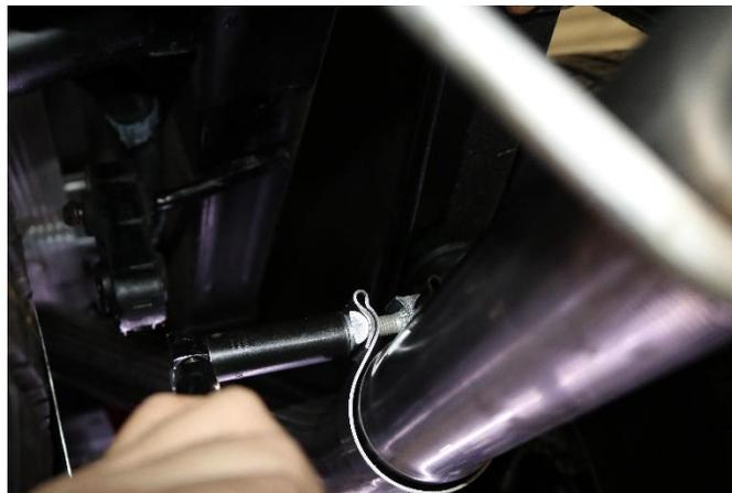
**21.** Visually inspect the exhaust system position, alignment, clamp orientation & position and exhaust system clearances. Make any adjustment necessary at the slip joints.
