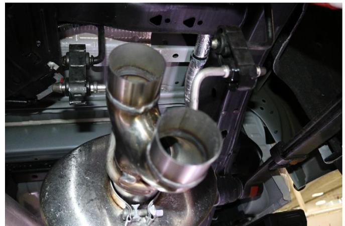
**10.** Insert the hangers on the Y-Pipe Assembly into the factory hanger grommets as shown.
