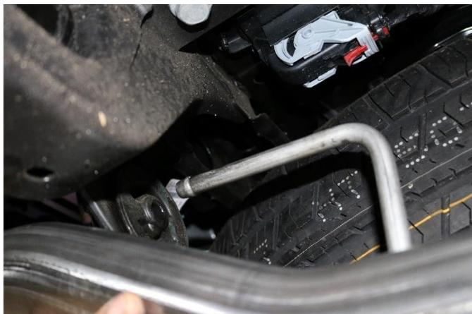
**18.** Insert the hanger on the passenger side rear tailpipe into the hanger grommet on the vehicle.
