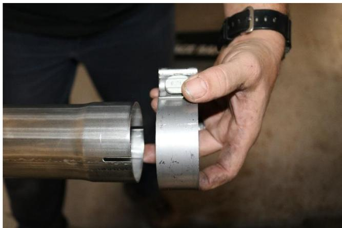
**17.** Insert a TORCA 2.5" clamp into the expanded and notched end of the passenger side rear tailpipe as shown.
