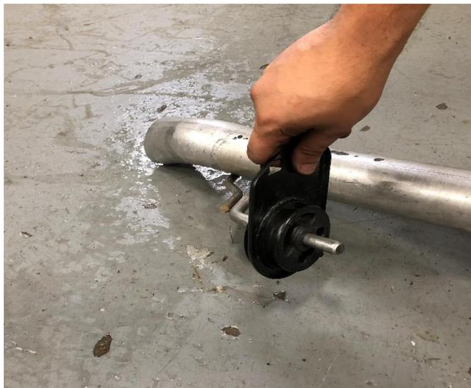
**13.** Remove the factory grommets from the driver's side tail pipe hanger and reattach it to the frame using a 13mm socket.
