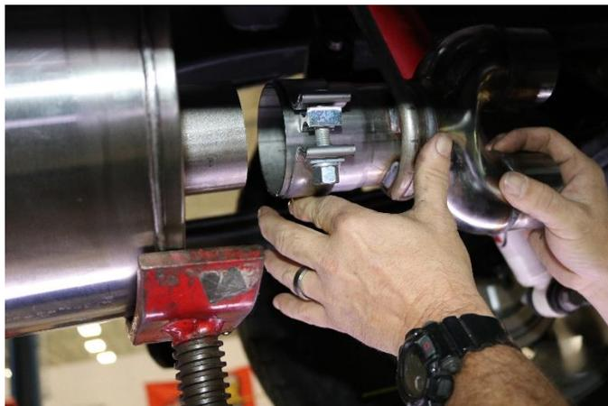
**9.** Slide the Y- Pipe Assembly into the side of the muffler supported by the stand as shown.
