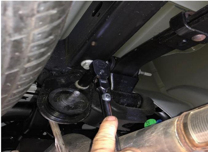
**9.** Disconnect the factory grommet from the frame using a 13mm socket on the driver's side tailpipe.
