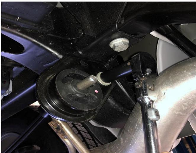
**11.** Disconnect the factory grommet from the frame using a 13mm socket on the passenger side tailpipe.
