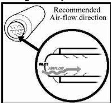
4. Install the **Muffler** and **4" Band Clamp** over the **Extension Pipe/s**. Refer to the figure on the left for correct **Muffler** orientation.
