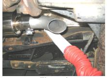
3. Loosely install the **Turn Down** connecting it to the **Muffler** outlet with the 2 ½" **Hanger Clamp**. Install the **Hanger Assembly** to the 2 ½" **Hanger Clamp** and to an existing hole in the frame using the fasteners provided. **Refer to Figures 6 &7**.
