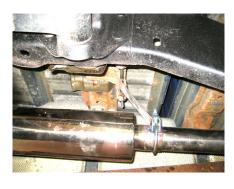
2. Install the **Muffler** onto the **Extension Pipe** using the **Hanger Clamp** provided. Then install the 2 ½"Hanger Clamp into the factory rubber insulator. Do not tighten the clamp at this time. **Refer to Figure 5**.
