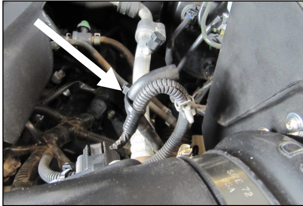
13. On 4WD models: Secure the differential breather to the MAF harness with the 8" Zip Tie. Trim off the excess.
