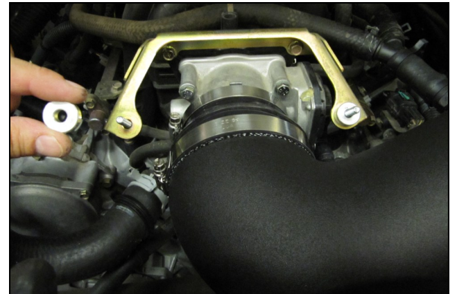
15. Reinstall the bracket onto the intake manifold and place a Spacer (#13) onto each 6mm bolt.
