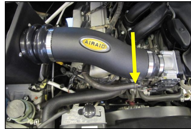
39. Install the Airaid Intake Tube onto the Cold Air Box and the throttle body, align and tighten all four of the Clamps. Reconnect the Mass Air Flow sensor. Connect the factory crank case breather line to the 3/8 Barbed Elbow on the Intake Tube
