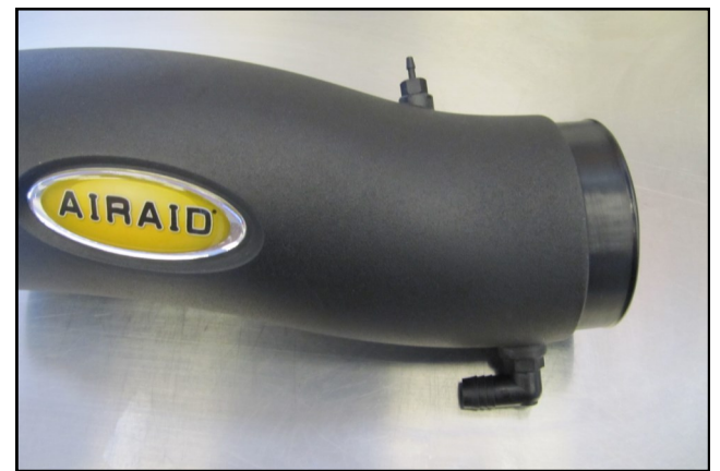
37. Install the 1/8" and 3/8" barbed fittings (#s 13 and 14) into the Airaid Intake Tube. Apply the Airaid Bubble Decal onto the Intake Tube as shown.
