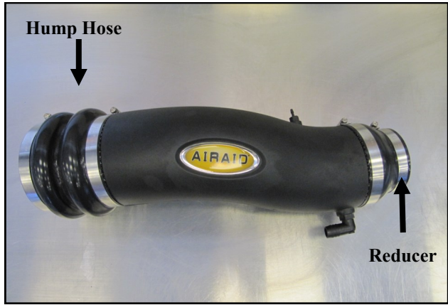
38. Slide the Hump Hose (#7), and two #68 Hose Clamps (#25), onto the Intake Tube as shown. Slide the Reducing Coupler (#8) and the #48 (#23) and #64 Clamps (#24) on the other end of the Intake Tube. Leave the Clamps loose for now.
