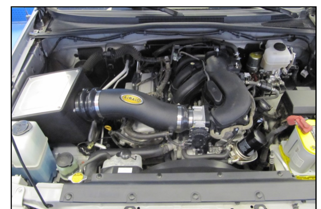
43. Double check your work! Make sure there is no foreign material in the intake path. Make sure all clamps, hoses, bolts, and screws are tight. Double check the hood clearance! Reconnect the negative battery cable!
