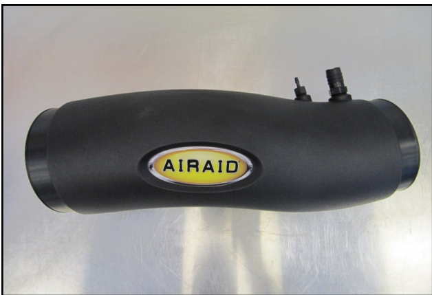
9. Install the 1/8" and 3/8" barbed fittings into the Airaid Intake Tube as shown. Apply the Airaid Decal onto the Intake Tube.
