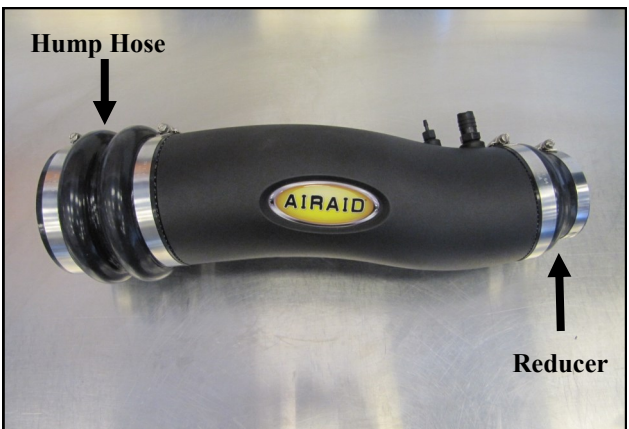
10. Slide the Hump Hose, and two #68 Hose Clamps onto the Intake Tube as shown. Slide the Reducing Coupler and the #48 and #64 Clamps on the other end of the Intake Tube. Leave the Clamps loose for now.
