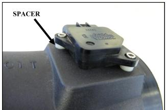
**8.** Transfer the Mass Air Flow sensor from the factory airbox, into the Airaid Intake tube and secure using the two #8 Spacers (#18) and 8-32 Socket Head screws (#22). **Do not use the factory screws.**
