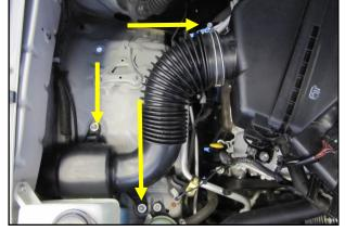
**2.** Loosen the clamp on the factory intake tube and remove the two 8mm bolts securing the other end on the inner fender. Slide the intake tube out from the inner lender hole and set it aside.
