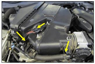
3. A.) Disconnect the Mass Air Flow meter.B.) Pry the wire harness anchor out of the airbox.
