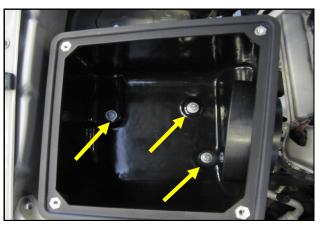
7. Mount the Cold Air Box onto the CAB Mounts using the three 8mm Bolts (#14) and 5/16 Flat Washers (#15)
