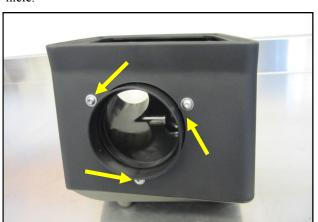
7. Mount the Filter Adapter (#5) to the Cold Air Box, as shown, using three 1/4-20 x 1/2" Button head Bolts (#16) and 1/4" Flat Washers (#17).
