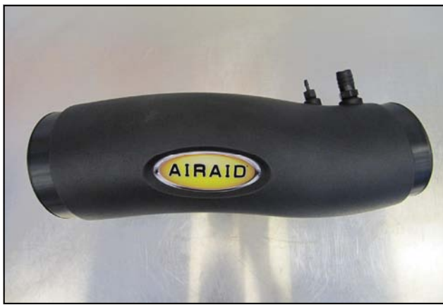
9. Install the 1/8" and 3/8" barbed fittings into the Airaid Intake Tube as shown. Apply the Airaid Decal onto the Intake Tube.
