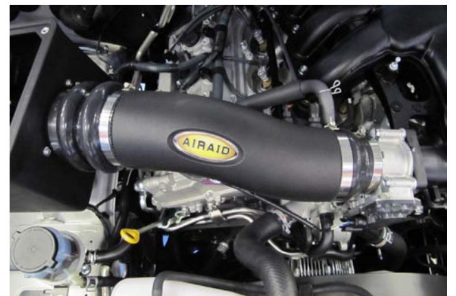
11. Install the Airaid Intake Tube onto the Cold Air Box and the throttle body, align and tighten all four of the Clamps. Reconnect the Mass Air Flow sensor.
