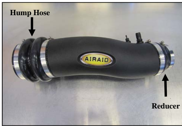
10. Slide the Hump Hose, and two #68 Hose Clamps onto the Intake Tube as shown. Slide the Reducing Coupler and the #48 and #64 Clamps on the other end of the Intake Tube. Leave the Clamps loose for now.
