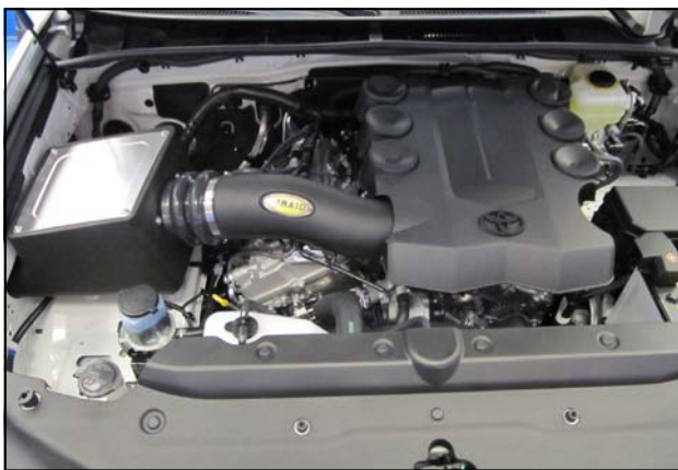
16. Double check your work! Make sure there is no foreign material in the intake path. Make sure all clamps, hoses, bolts, and screws are tight. Double check the hood clearance!
