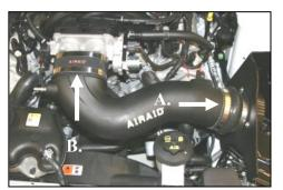
**14.** A.) Install the tube into the hump hose. B.) Now slide the oval coupler onto the throttle body. Tighten the remaining two hose clamps, and re-connect the mass air sensor, from step #2.
