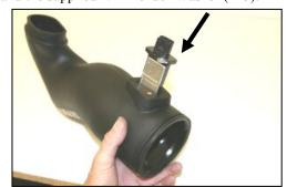
**12.** Align the two slots in the tubes, and install the factory mass air sensor removed from step #5. Make sure the screw holes line up, then install the two supplied button head screws. (#11).
