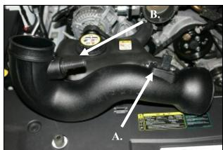
12. A.) Install the MAF sensor removed in step #5, into the Airaid Intake Tube (#2). Use the two supplied 8-32 button head bolts (#10), to securely fasten the MAF sensor. Do Not Use The Factory Screws!
