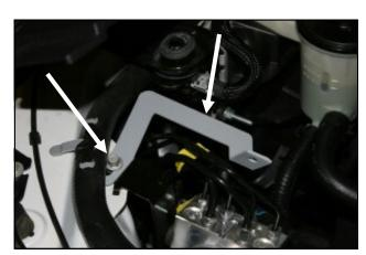
7. Lift up the corner of the plastic trim from step #6 to gain access to the bolt that secures the bracket for the anti lock brake manifold. Remove the bolt and install the front bracket (#17) as shown. Replace the factory bolt and leave it just snug for now.
