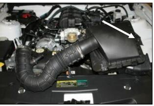
**3.** Remove the complete intake system as an assembly. Remove the factory grommet, and steel sleeve from the factory airbox for reuse in step #8.
