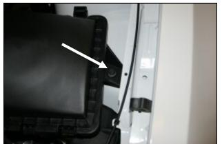
**2.** Remove the bolt that holds the factory airbox to the driver's side inner fender. (Save this bolt for later use in step #9).
