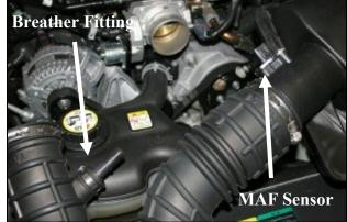
**5.** Using the supplied #20 torx bit, remove 2 factory screws, and remove the **MAF** sensor from the factory tube. (Save the **MAF** sensor for reinstallation in step #12). Next, using a pair of side cutters, remove the metal band that holds the plastic breather fitting into the factory air intake tube . Now remove the fitting from the tube, and save it for reinstallation in step #12.
