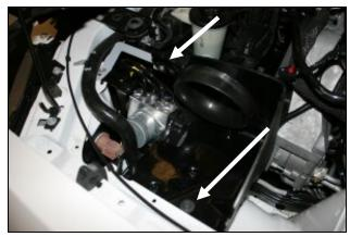
9. Install the CAD into the vehicle aligning the locating pins on the bottom of the CAD into the factory grommets in the fender. Reinstall the factory bolt from step #2 into the steel sleeve and grommet. Next install the 1/4-20x5/8" hex bolt (#14) thru one 1/4" flat washer (#9), thru the CAD, and thru the bracket securing it with one 1/4" serrated nut (#15). Adjust for fit and then tighten the bolt on the anti lock brake bracket.
