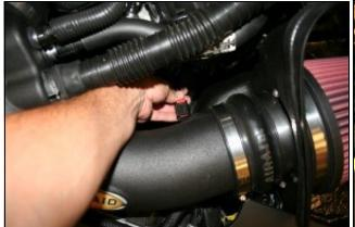
located in the lower back side of the intake. Slide the locking tab back into the connector.
