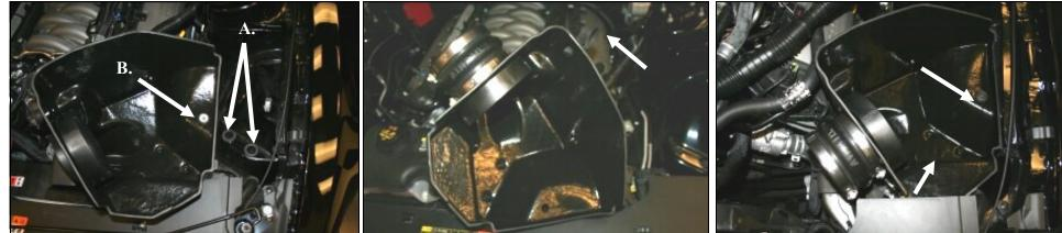
7. Transfer the factory air box mounting grommets. A) Locate and remove the Two Lower air box mounting grommets, and install them in the inner fender. B) Remove the Upper air box mounting grommet and steel sleeve, and re-install into the Airaid CAB.
