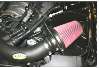
12. A) Install the Airaid Premium Filter (#1) onto the filter adapter and tighten the hose clamp. B) re install the Resonator tubing into the factory Stand off.
