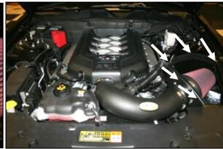
13. Reconnect the Mass Air Flow sensor, which is now 14. Install the Weather Strip (#9) onto the CAB with the contoured edge going away from the filter. Start at the front of the vehicle and work your way back. Replace the engine cover.
