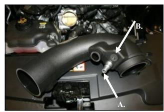
4. Install the Grommets and Fittings into the Airaid intake 5. Using the supplied Torx driver, remove the MAF sen- 6. Install the filter adapter (#8) using three 1/4-20 button tube (#2). A) All models will require the use of the 5/8" sor from the Factory airbox and create the Tube assem- head bolts (#10), and flat washers (#11) into the Airaid Fitting (#19) and the 5/8"Grommet (#20). B) Automatic bly.
