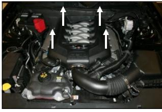
**Disconnect The Negative Battery Terminal!** 1. Remove the Engine cover by simply lifting up, and set aside.
