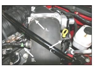
2. A.) Loosen the factory intake tube hose clamp on the throttle body. B.) Push the GREEN tab on the breather hose connector and disconnect it from the factory intake tube. C.) CAREFULLY disconnect the vacuum line from the factory intake tube.
