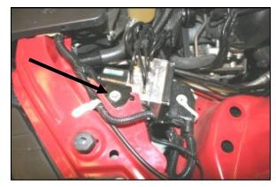
**6.** Using a 10mm socket, remove and save the bolt from the top of the anti-lock brake bracket. It will be re-installed later in step #13.
