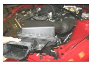
**3.** Remove the complete factory intake system from the vehicle.
