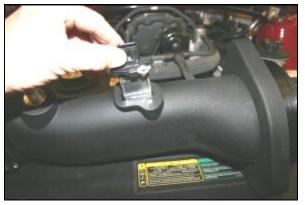
9. Install the Mass Air Flow sensor removed in step #5, into the Airaid Intake Tube using the provided 8 -32 x 3/8" button head screws (#8). Make sure the arrow on the sensor is pointing towards the throttle-
