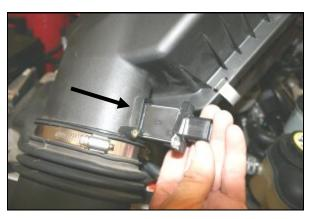
5. Using the provided #20 torx bit, remove two factory screws and the Mass Air Flow sensor from the factory airbox lid. Note the direction of the sensor for proper re-installation later. (Save the mass air sensor for re-installation in step #9, the factory screws will not be re-used).
