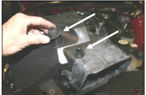
4. Remove the two factory grommets from the bottom of the factory airbox and replace them back into the holes in the inner fender. They will be used to guide the Airaid Cool Air Dam to the correct location in the vehicle.
