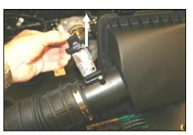
**5.** Using the supplied #20 torx bit, remove 2 factory screws, and remove the MAF sensor from the factory tube. (Save the MAF sensor for reinstallation in step #12).
