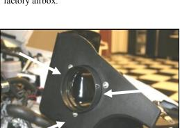
7. Install the air filter adapter (#5) into the Cool Air Dam (#6) as shown, using 3 button head bolts (#8) and ½" flat washers (#9).
