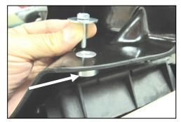
7. Install the air filter adapter (#5) into the Cool Air Dam (#7) as shown, using 3 button head bolts (#9) and <sup>1</sup>/<sub>4</sub>" flat washers (#10).
