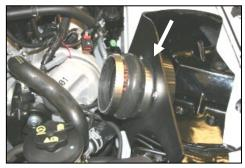
**10.** Install the hump hose (#5) on the filter adapter (#6), with two #72 hose clamps (#13). Tighten <u>only</u> the clamp next to the **CAD**.
