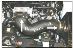
**15.** A.) Install the tube into the hump hose. B.) Now slide the oval coupler onto the throttle body. Tighten the remaining two hose clamps, and re-connect the mass air sensor, from step #2.
