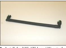
**18.** Install the 3/8"x12" hose (#8) onto the factory breather ends as shown.
