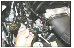
1. Disconnect negative battery cable. PLEASE READ #22 ON THE BACK PAGE!! Push the green plastic tabs, and remove breather hose from vehicle. (Save for later use).
