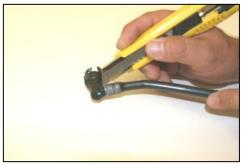
**17.** <u>VERY CAREFULLY !</u> Using a razor blade, cut the plastic tube off both of the factory breather hose ends as shown.
