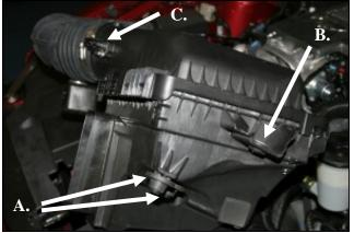
**3.** Grab the airbox and tube and roll it forward while lifting up to dislodge it from the intake scoop. Remove the assembly from the vehicle. A.) Remove the two factory grommets and then replace them back into the two holes in the inner fender. B.) Remove the steel sleeve and grommet and save for reinstallation later. C.) Using the provided #20 Torx bit, remove the two screws and the
