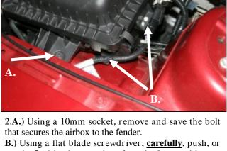
pry the 5 wiring loom anchors from the factory airbox.
