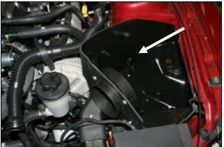
scoop provision in the CAB aligns with the factory scoop, and the two locating pins on the bottom align with the factory grommets. Next reinstall the factory bolt that was removed in step #2 thru the steel sleeve and grommet and into the inner fender. Make sure that the wiring harness is not pinched under the CAB.
