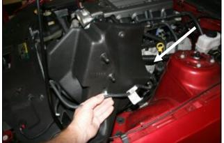
their respective holes starting at the back of the CAB with the two hole anchor and work your way underneath and towards the front. The last anchor nearest the MAF sensor is not anchored.
