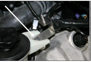
11. Install the bracket assembly from step #10 as shown. 12.A.) Install the oval coupler onto the intake tube This bracket and 6mm bolt will secure the power steering using two #72 hose clamps (#15). Leave the clamps loose reservoir and replaces the stud removed in step #9.
