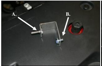
10.A.) Thread the 1/4-20 hex bolt (#13) into the resonator bracket (#21) and tighten as shown. **B.**) Slide the 6mmx12mm (#15) hex bolt thru one flat
