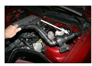
**6.** Grab the resonator tube between the diaphragm and the firewall and pull up and out to disconnect it from the firewall. Remove the complete resonator assembly from the vehicle.
