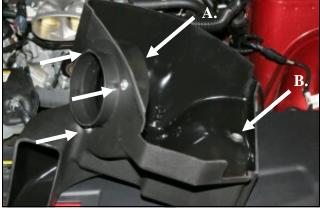
4. A.) Install the filter adapter (#7) using three 1/4-20 5. Turn the CAB so that the bottom faces the left fender 6. Install the CAB into the vehicle making sure that the button head bolts (#11), and flat washers (#10) into the as shown. Now reinstall the wiring loom anchors into Airaid Cool Air Box (CAB) (#3) as shown. B.) Reinstall the small grommet and sleeve (removed in step #3) into the hole in the CAD.
