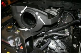
**6.** Install the filter adapter using three 1/4-20 button head bolts, and flat washers into the Airaid Cool Air Box
