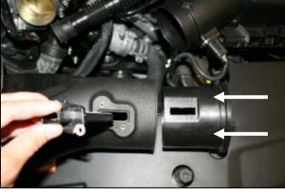
A) Slide the Modular Venturi Tube into the Airaid intake tube making sure to align the two slots for the MAF sensor. B) Install the MAF sensor into the intake tube using two provided 8-32x3/8" screws.
