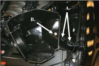
Locate and remove the Two Lower air box mounting #72 hose clamps as shown. Leave the two hose clamps move the Upper air box mounting grommet and steel factory air box into the CAB. sleeve, and re-install into the Airaid CAB.
