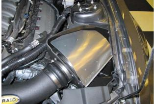
13. Reconnect the Mass Air Flow sensor, which is now 14. Mount the Rain Shield onto the Airbox as shown 15. Install the Weather Strip onto the CAB with the conusing the 1/4-20 Button Head Screws and Washers. toured edge going away from the filter. Start at the front NOTE: Installation of the Rain Shield is optional but of the vehicle and work your way back. Replace the enhighly recommended for vehicles with Power Dome gine cover. hoods with heat extractors.
