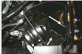
9. Install the CAB into the vehicle. Make sure that the Air inlet of the CAB aligns with the factory duct, and the two locating pins on the bottom align with the factory grommets. Next reinstall the factory bolt that was removed in step #3 thru the steel sleeve and grommet and into the inner fender.
