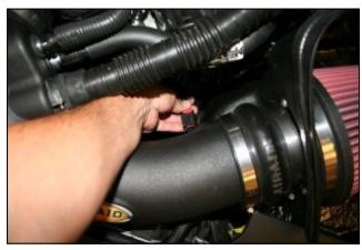
located in the lower back side of the intake. Slide the locking tab back into the connector.
