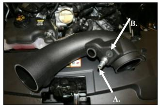
4. Install the Grommets and Fittings into the Airaid intake 5. Using the supplied Torx driver, remove the MAF sentube. A) All models will require the use of the 5/8" Fit- sor from the Factory airbox and create the Tube assemting and the 5/8"Grommet. B) Automatic transmission bly. equipped vehicles will also use the 3/8" Fitting and 3/8" Grommet. Manual transmission vehicles will not need the 3/8" components and will use the Blind Grommet.
