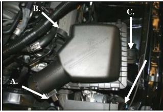
3. A) Slide the red tab, and disconnect the wiring harness from the Mass Air Flow sensor (MAF). Carefully pry the harness anchor from the air box using a screwdriver. B) Separate the resonator tube from the stand off attached to the Air box lid. C) Using a 10mm socket, remove the bolt securing the air box to the inner fender and remove the air box assembly. This bolt will be reused in
