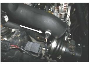
**11.** On 1999-01 Models, Carefully install the factory intake temp sensor into the grommet in the Airaid Intake Tube.
