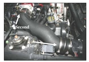
**12.** Install the Airaid Intake Tube into the hump hose first, and then onto the throttlebody. Adjust for fit, and then tighten the two remaining hose clamps. Reconnect the crankcase breather hose to the 5/8"x 3" hose, and connect the idle bypass hose to the 3/4" barbed fitting. Now reinstall the **MAF** sensor onto the **MAF** housing using the factory screws.
