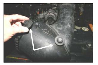
**4.** Remove the two factory grommets from the bottom
