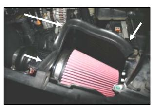
**13.** Install the supplied weather strip (#7) onto the top of the **CAD** starting at the fender and working your way towards the radiator.
