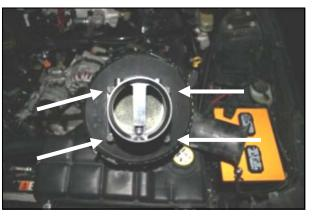
5. Remove the four bolts that hold the **MAF** housing to
