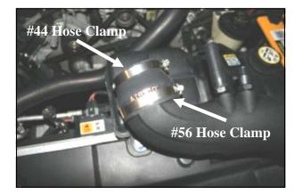
**8.** Install the reducer coupler (#4) onto the throttlebody end of the Airaid Intake Tube using the #56 hose clamp (#14) on the tube end, and the #44 hose clamp (#13) on the small end. Tighten *only* the large #56 clamp at this time. Air Dam (#6) using four 6mmx25mm bolts (#8), four lock washers (#10), two MAF gaskets (#12), and one velocity stack (#3). Refer to the line drawing at the top of this page for the proper sequence of how to install the parts.
