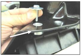
8. Slide the Aluminum Spacer (#17) underneath the CAD and into the hole as shown. Secure the CAD to the inner fender using the OEM bolt from step # 2 and the supplied 1/4" Fender Washer (#18).
