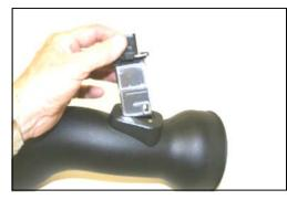
12. Install the MAF sensor from step #5 into the Airaid Intake Tube. Use the two supplied 8 -32 button head bolts (#10), to securely fasten the MAF sensor.
