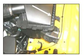
2. Remove bolt that holds the factory airbox to the fender. (Save bolt for later use in step #7).
