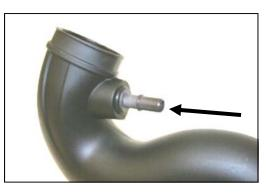
**11.** Install the factory fitting from step #7 into the grommet (#16) from step #10.
