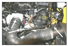
**Disconnect negative battery cable.** 1. A) Loosen hose clamp on throttle body. B). Push green tab, and disconnect breather hose at the factory intake tube. C) Slide red tab, and disconnect the Mass Air Flow sensor wiring harness.
