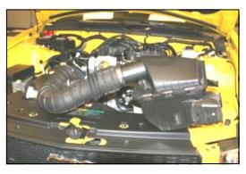
3. Remove the complete intake system as an assembly.
