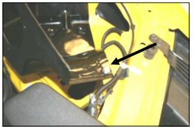
**9.** If your vehicle has the optional anti-lock brakes, remove the bolt from the bracket under the CAD, and reinstall it thru the hole in the front of the CAD. (See arrow). If your vehicle does not have this bracket, install the supplied 1/4" bolt (#14), two 1/4" washers (#9), and 1/4" Nylock nut (#15) thru the CAD and sheet metal, and tighten.
