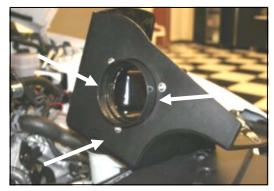
Install the air filter adapter (#5) into the 7. Cool Air Dam (#6) as shown, using 3 button head bolts (#8) and 1/4" flat washers (#9).
