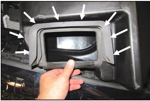
10. Transfer the factory airbox coupler from the OEM airbox inlet into the Airaid Cold Air Box, or C.A.B.(#3).
