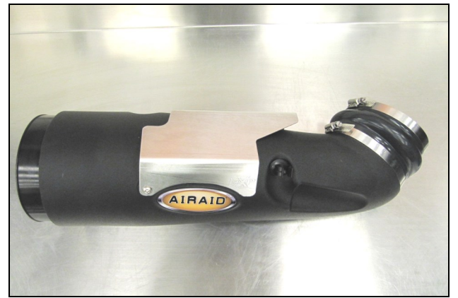
12. Slide the Hump Hose (#5) and Clamps (#14) onto the Airaid Intake Tube. Leave the clamps loose for now.
