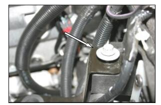
**3.** Remove one bolt from the factory airbox mounting plate, and save it for reinstallation in step #8.
