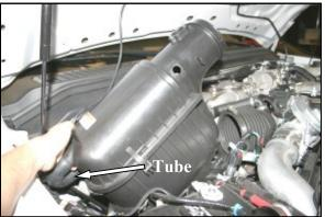
**2.** Remove the factory airbox and tube from the vehicle as an assembly, by pulling straight up on the box. It is only held in place by grommets, no bolts.
