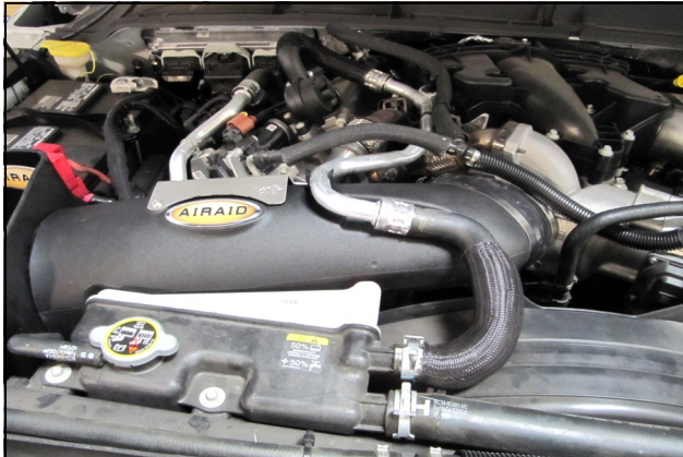
13. Install the Airaid Intake Tube assembly. A.) Slide the Tube, Hump Hose end first, under the coolant line and onto the turbo inlet. B.) Insert the Filter end of the Tube into the CAB.
