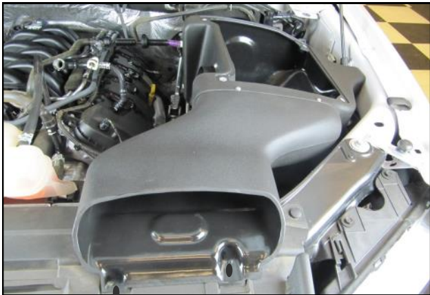
10. Place the Airaid air Box/Inlet assembly into the inner fender area of the vehicle as shown.
