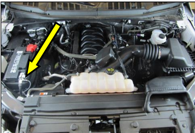
1. Disconnect the negative battery terminal.
