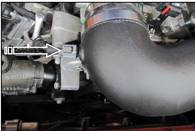
14. Reconnect the air temperature sensor.
