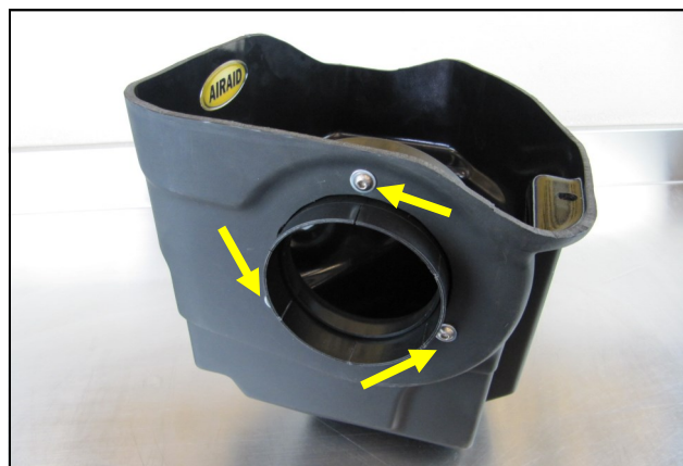
4. Install the Filter Adapter onto the Cool Air Box using the three 1/4" Button Head Screws and 1/4" Flat Washers, (#s 8&9). Apply the Airaid Bubble Decal inside the Air-box as shown.
