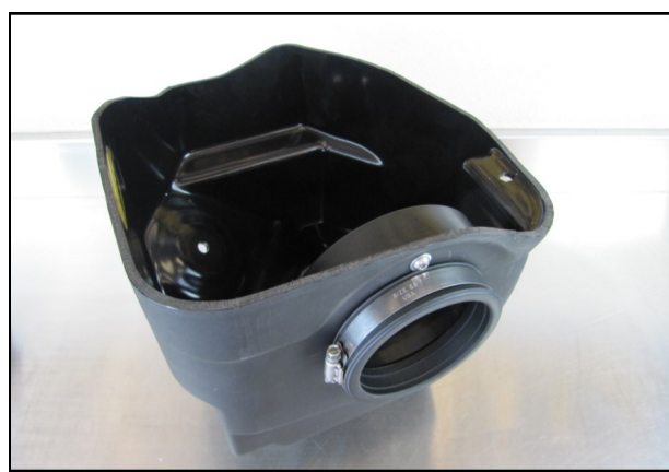
5. Slide the Coupler and Clamp onto the Filter Adapter as shown. Do not tighten the Clamp at this time.
