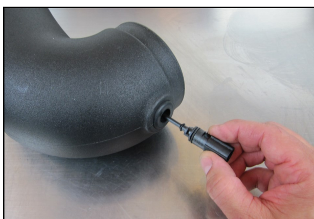
8. Insert the 9/16" Grommet into the Airaid Intake tube and shown. Transfer the air temperature sensor from the factory intake tube into the Airaid Intake Tube.
