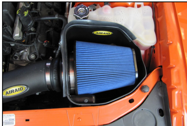
17. Install the Weatherstrip onto the top edge of the Air Box with the contour rolling away from the Filter.
