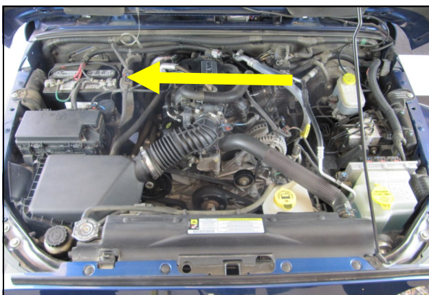
1. Disconnect The Negative Battery Terminal! It's recommended to allow the engine to fully cool down before starting the intake installation.
