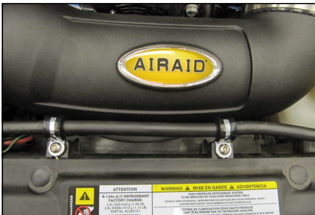
16. Secure the coolant line to the fan shroud using the two Adel Clamps, 6 mm Bolts, and 1/4" Flat Washers.
