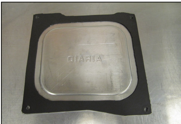
19. Place the Gasket onto the underside of the Air Box Lid and peel off the protective film. Mount the lid on the Air Box using four 1/4-20 x 1/2" Button Head Bolts, and 1/4" Flat washers.
