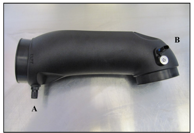
12. A.) Install the 5/8" Barbed Fitting into the threaded 3/8 hole in the side of the Airaid Intake Tube. B.) Transfer the air temp sensor from the factory intake into the Airaid Intake Tube and secure it using the #8-32 x 1/2" Button Head Bolt and #8 Fender Washer.
