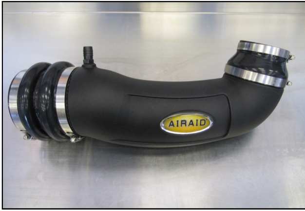
13. Slide the Double Hump Hose, and two #72 Hose Clamps, onto straight end of the Tube. Slide the Silicone Reducer and the #48 and #64 Clamps on the 90 deg. bend of the Intake tube. Leave the Clamps loose for now. Apply the Airaid Decal to the Tube as shown.
