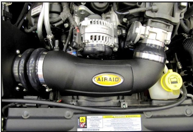
14. Install the Airaid Intake Tube onto the Cold Air Box and throttle body, align, and tighten all four of the Clamps. Reconnect the air temp sensor.
