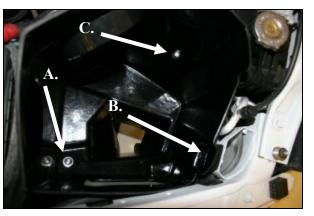
9. Install the CAB into the vehicle as shown. A.) Install the 3/8" button head bolt (#17) and flat washer (#18) thru the CAB and into the well nut. B.) Install the 6mm x 25mm hex bolt (#15) and flat washer (#10) thru the CAB and into the captured nut in the fender. C.) Install the 5/16" bolt (#11) flat washer (#12), and flange nut (#13) thru the CAB and L-bracket. Tighten all mounting bolts at this time.
