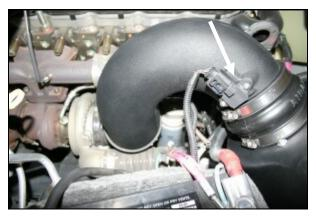
**11.** Install the Airaid Intake Tube (#2) into the factory turbo elbow and then into the hump hose. Adjust for fit, and then tighten all three hose clamps. Reinstall the intake temperature sensor into the Airaid Intake Tube using two 8-32 button head screws (#7) and #8 flat washers (#8). **Do Not Use The Factory Screws!**
