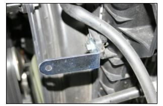
6. Install the L-bracket (#20) onto the radiator shroud using one M8 x 30mm bolt (#14) and one flat washer
