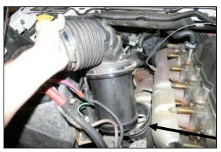
3. Loosen the hose clamp that secures the factory intake tube assembly to the rubber elbow on the turbo inlet, and remove the assembly from the vehicle.
