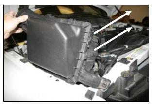
2. Slide the flexible intake tube off of the factory airbox lid and then rock the factory airbox assembly side to side to release it from the mounting grommets, and remove it from the vehicle.
