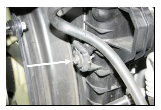
5. Using a 13mm socket remove one bolt that secures the fan shroud to the radiator on the passenger side of
