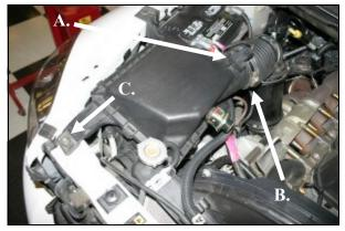
1. Disconnect the negative battery cables. A.) Using the provided T-20 torx bit, remove the two temperature sensor mounting bolts and the sensor from the factory intake tube (set aside for reuse). **B**.) Loosen the hose clamp where the flexible tube connects to the factory airbox lid. C.) Using a 10mm socket, remove the nut that secures the factory airbox to the radiator mount.
