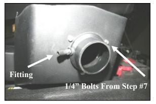
**8.** Install the 1/4" NPT x 1/2" barbed fitting (#17) into the filter adapter as shown.
