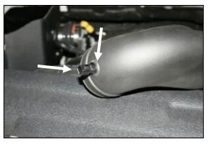
**15.** Install the supplied grommet (#14) into the hole in the Airaid Intake tube(#2). Next carefully install the factory intake air temperature sensor into the grommet
