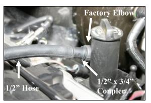
11. Remove the factory hard plastic breather tube from the rubber elbow behind the oil filler neck and then install the supplied 1/2" x 3/4" plastic reducing coupler (#18), into the factory rubber elbow as shown. Next, connect the supplied 1/2" x 22" hose (#7) to the coupler.
