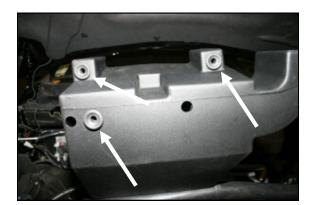
**4.** Rock the airbox back and forth as you are lifting it straight up to remove it from the vehicle. It is only held in by grommets.
