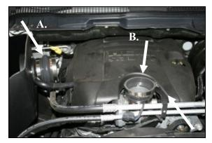
**14.** A.) Install the supplied hump hose (#5) onto the filter adapter using one #60 hose clamp (#12) and one #64 hose clamp (#13). B.) Install the reducing coupler (#4) onto the throttlebody using one #52 hose clamp (#11) and one #60 hose clamp (#12). Leave the clamps loose for now.
