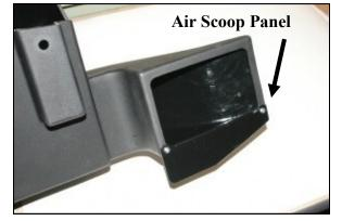
**9.** Install the air scoop panel (#20) onto the scoop of the **CAB** using two #8 x 3/8" self tapping screws (#21) as shown.
