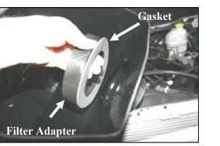
**7.** Install the adapter gasket (#19) and filter adapter (#6) into the **CAB** using three 1/4-20 x 5/8" bolts (#9) and flat washers (#10) as shown. *Refer to the line drawing above for reference.*
