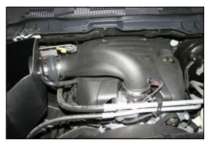
**16.** Install the Airaid Intake tube into the hump hose first, and then into the coupler on the throttlebody. Tighten all four hose clamps, and then reconnect the intake air temperature sensor wiring harness.
