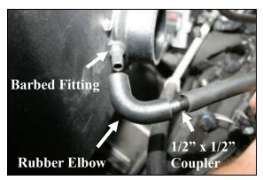
**12.** Install the supplied 1/2" x 1/2" plastic coupler (#16) into the 1/2" hose from step #11. Next connect the 1/2" rubber elbow (#15) between the 1/2" connector and the barbed fitting on the filter adapter.
