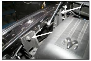
**3.** Using a 13mm socket, remove the two bolts that hold the air cleaner mount to the inside right fender. Save them for reinstallation in step #10.
