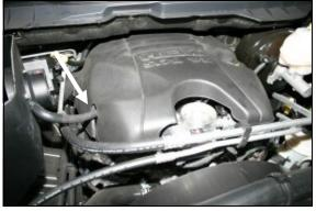
**13.** Reinstall the factory beauty cover making sure that the grommets are aligned with the grommet posts and that the crankcase breather hose is aligned in the slot on the side of the cover.
