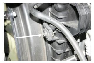
**5.** Using a 13mm socket remove one bolt that secures the fan shroud to the radiator on the passenger side of the vehicle.
