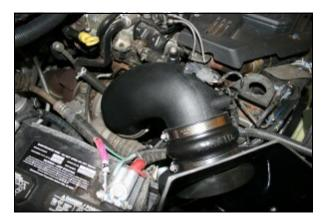
11. Install the Airaid Intake Tube (#2) into the factory turbo elbow and then into the hump hose. Adjust for fit, and then tighten all three hose clamps. Reinstall the intake temperature sensor and Mass Air Flow sensor into the Airaid Intake Tube using three 8-32 button head screws (#7) and #8 flat washers (#8). **Do Not Use The Factory Screws!** Reinstall the factory wiring harness anchor into the hole in the Airaid Intake Tube.
