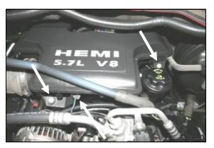
2. Squeeze the tab on the connector and disconnect the intake temperature sensor wiring harness on the front of the resonator. Next remove the two bolts that secure the resonator to the engine. Lift the resonator up at the front, and remove it from the vehicle.
