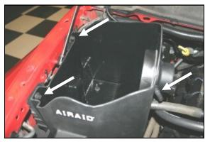
**9.** Install the **CAD** into the vehicle by aligning the grommets over the locating pins on the factory airbox mount. Reinstall the factory bolts in the fender that were removed in step #4. Next install the 1/4"NPT x 1/2" barbed fitting (#19) into the **CAD**.
