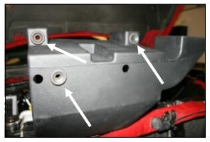
7. Install the three grommets removed in step # 6 into the bottom of the Airaid Cool Air Dam (CAD)(#3) at the locations shown here.
