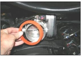
**3.** Remove the factory seal from the throttle body.
