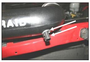
**11.** Install the supplied grommet (#13) into the Airaid intake tube(#2). Next, *carefully* install the factory air intake temperature sensor into the grommet in the tube. Make sure it is fully seated into the grommet.
