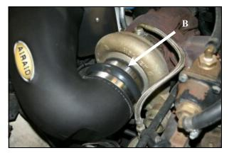
7. A) Install the CAB and Tube assembly onto the turbo inlet first, then rotate the assembly downward onto the inner fender studs. B) Secure the Silicone reducer to the turbo inlet using the # 64 Clamp (#13).
