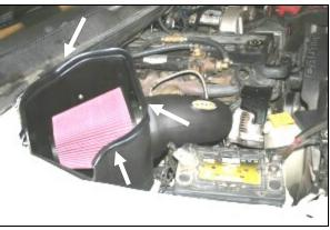
**9.** Install the Airaid Premium Filter (#1) onto the Intake tube as shown and tighten the clamp. Install the Weatherstrip (#6) onto the top edge of the **CAB** staring from the front and work your way back
