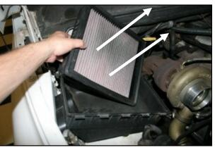
**2.** Remove the factory air filter from the lower half of the factory airbox.
