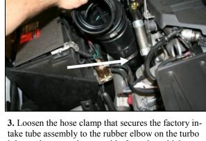
inlet, and remove the assembly from the vehicle..
