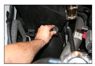
7. Install the Two supplied well nuts (#14) into the factory airbox mounting holes as shown.
