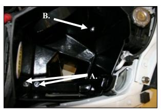
9. Install the CAB into the vehicle as shown. A.) Install the 3/8" button head bolts (#15) and flat washer (#16) thru the **CAB** and into the well nuts. **B**.) Install the 5/16" bolt (#11) flat washer (#12), and flange nut (#13) thru the CAB and L-bracket. Tighten all mounting bolts at this time. Apply the Airaid Decal in the Airbox as shown.
