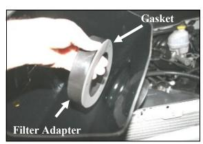
7. Install the adapter gasket (#19) and filter adapter (#6) into the **CAB** using three 1/4-20 x 5/8" bolts (#9) and flat washers (#10) as shown. *Refer to the line drawing above for reference*.
