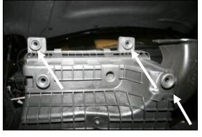
**5.** Remove and save three grommets from the bottom of the factory airbox. They will be reused in step #6.
