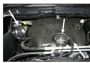
**14.** A.) Install the supplied hump hose (#5) onto the filter adapter using one #60 hose clamp (#12) and one #64 hose clamp (#13). B.) Install the reducing coupler (#4) onto the throttlebody using one #52 hose clamp (#11) and one #60 hose clamp (#12). Leave the clamps loose for now.
