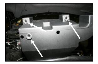
**6.** Install the three grommets removed in step #5 into the bottom of the Airaid Cool Air Box (CAB) (#3) at the locations shown here.
