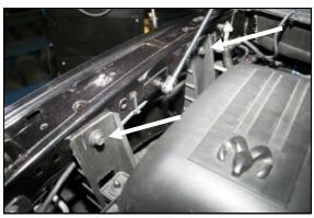
**3.** Using a 13mm socket, remove the two bolts that hold the air cleaner mount to the inside right fender. Save them for reinstallation in step #10.
