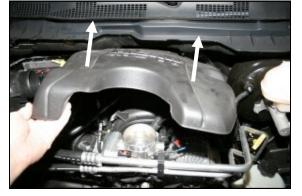
**2.** Lift up the front of the engine beauty cover, and then pull it towards you to remove it from the vehicle. It is only held in position by rubber grommets.
