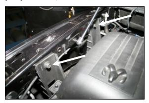
**3.** Using a 13mm socket, remove the two bolts that hold the air cleaner mount to the inside right fender. Save them for reinstallation in step #9.
