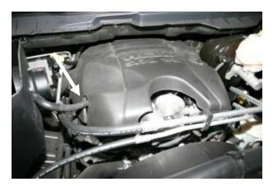
12. Reinstall the factory beauty cover making sure that the grommets are aligned with the grommet posts and that the crankcase breather hose is aligned in the slot on the side of the cover.
