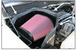
11. Install the Airaid Premium Filter (#1) onto the filter adapter and tighten the clamp. Next install the weather strip (#4) on the top of the CAB as shown. (Hint: Start at one end of the CAB and work your way towards the other end.)
