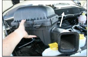
**2.** Rock the airbox back and forth as you are lifting it straight up to remove it from the vehicle. It is only held in by grommets.
