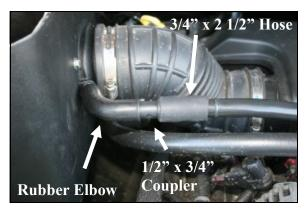
**10.** Install the supplied 3/4" x 2 1/2" hose (#11) onto the factory crankcase breather tube, and then insert the 1/2" x 3/4" barbed connector (#9) into the 3/4" hose. Next connect the 1/2" rubber elbow (#7) from the 1/2" barbed fitting on the filter adapter to the 1/2" x 3/4" connector. See the line drawing on the front page for reference.
