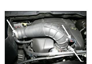
**13.** Reinstall the factory air intake tube. Reconnect the electrical connector to the temperature sensor, and then tighten both hose clamps.
