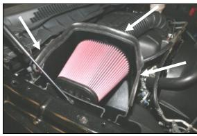
14. Install the Airaid Premium Filter (#1) onto the filter adapter and tighten the clamp. Next install the weather strip (#5) on the top of the CAB as shown. (Hint: Start at one end of the CAB and work your way towards the other end.)
