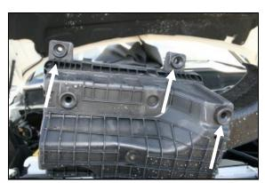
**3.** Remove and save three grommets from the bottom of the factory airbox. They will be reused in step #4.
