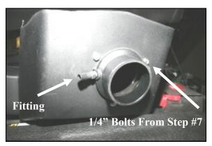
**8.** Install the 1/4" NPT x 1/2" barbed fitting (#9) into the filter adapter as shown.
