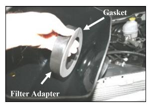
7. Install the adapter gasket (#12) and filter adapter (#3) into the **CAB** using three 1/4-20 x 5/8" bolts (#6) and flat washers (#7) as shown. *Refer to the line drawing above for reference*.
