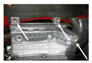
6. Remove and save three grommets from the bottom of the factory airbox. They will be reused in
