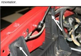
4. Using a 13mm socket, remove two bolts holding the airbox mounting bracket to the inner fender. These bolts will be reused in step #9.
