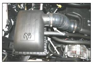
1. Disconnect the negative battery cable! Loosen the hose clamp on the flexible intake tube at the airbox lid. Disconnect the breather hose going into the factory airbox lid. Slide the flexible tube off of the lid and lift the airbox assembly straight up and out of the vehicle. 2003 Models: Disconnect the breather hose from the back of the
