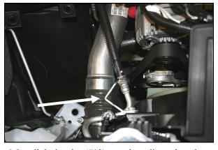
6. Install the bracket (#18) onto the radiator shroud as shown using the factory hardware. Leave the bolt slightly loose for now.
