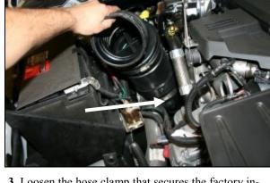
3. Loosen the hose clamp that secures the factory intake tube assembly to the rubber elbow on the turbo inlet, and remove the assembly from the vehicle..
