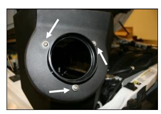
**8.** Install the filter adapter (#4) into the Cool Air Box, (CAB),(#3) using three 1/4" Button Head bolts (#9) and flat washers (#10) as shown.
