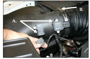
1. Disconnect the negative battery cables. A) Disconnect the air sensors on the upper half of the Factory Airbox, and detach the wire harness. B) Loosen the hose clamp that secures the factory intake tube assembly to the Airbox, unclip the Airbox lid, and remove the upper half of the factory airbox from
