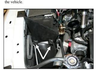
4. Remove the two Factory Airbox grommets and set aside. They will not be reused.
