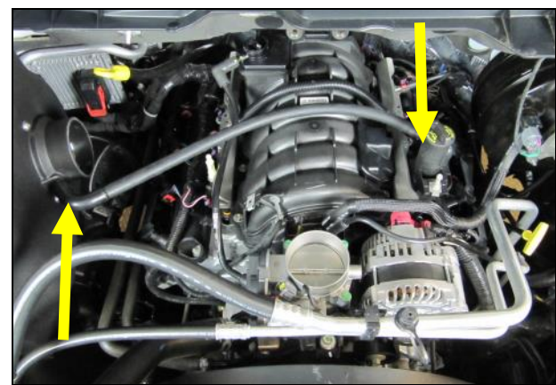
12. Install the Elbow side of the Airaid PCV line onto the Barbed Fitting on the Cool Air Box and connect the other side to the factory valve cover elbow.
