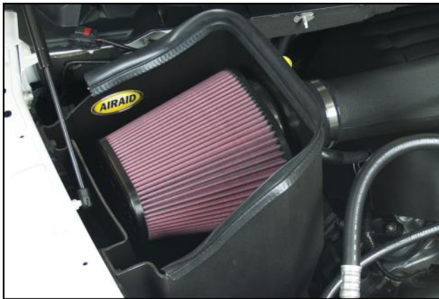
17. Install the Airaid Premium Filter onto the Filter Adapter inside the Cool Air Box. Install the Weatherstrip onto the Cool Air Box as shown, with the contour rolling away from the Filter. Complete the install by applying the Airaid Decal to the inside of the Airbox.
