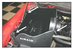
9. Install the CAD into the vehicle by aligning the grommets over the locating pins on the factory airbox mount. Reinstall the factory bolts in the fender that were removed in step #4. Next install the 1/4"NPT x 1/2" barbed fitting (#19) into the
