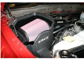
14. Install the Airaid Premium Filter (#1) onto the tube on the filter adapter and tighten the clamp. Next install the weather strip (#7) on the top of the Quick Fit Panel as shown. (Hint: Start at one end of the CAD and work your way towards the other end)
