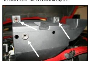
7. Install the three grommets removed in step # 6 into the bottom of the Airaid Cool Air Dam (CAD)(#3) at the locations shown here.
