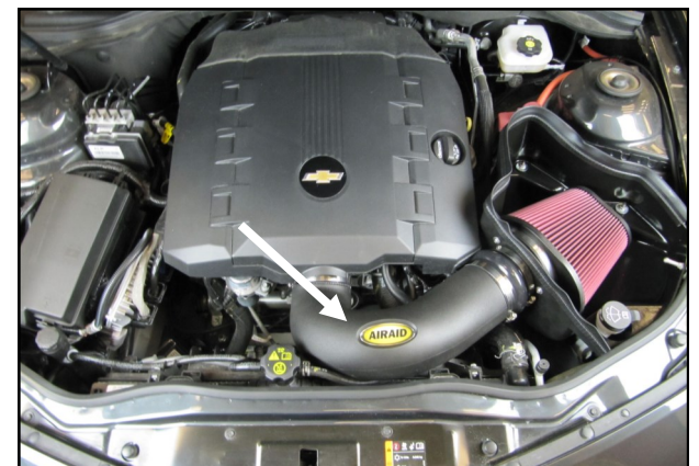
18. Double check your work! Make sure there is no foreign material in the intake path. Make sure all clamps, hoses, bolts, and screws are tight. Double check the hood clearance! Reconnect the negative battery cable. Apply the Airaid Decal onto the Intake Tube.
