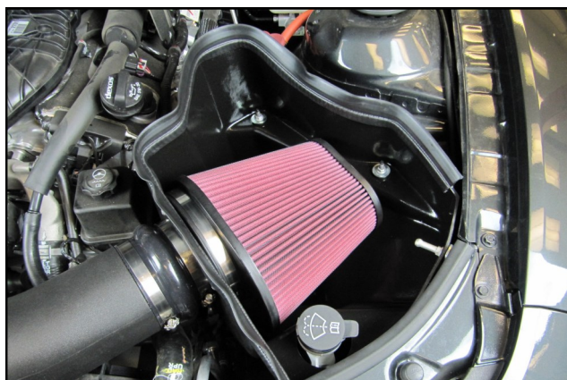
17. Install the Weatherstrip onto the Cool Air Box as shown, with the contour rolling away from the Filter. Reinstall the engine cover and oil fill cap.
