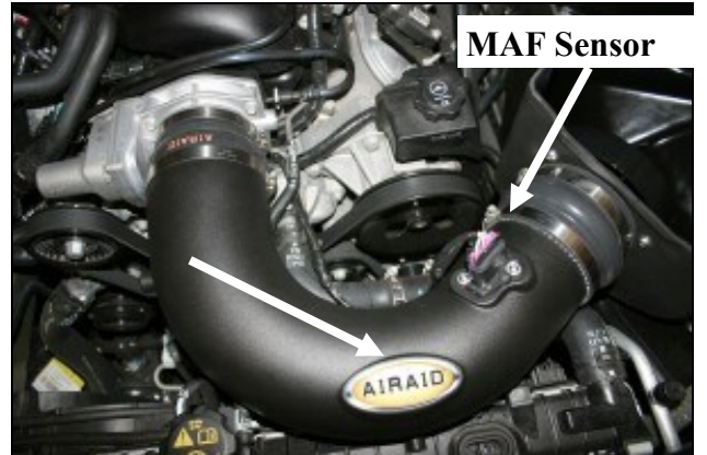
15. Install the Airaid Intake Tube (#2) into the hump hose first, and then into the reducing coupler. Adjust for fit, and tighten all four hose clamps. Next install the MAF sensor into the tube and secure it using two 8-32 x 3/8" button head screws (#20). Apply the Airaid Decal onto the Intake Tube as shown.
