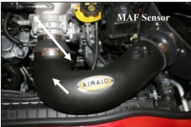
16. Install the Airaid Intake Tube (#2) into the hump hose first, and then into the reducing coupler. Adjust for fit, and tighten all four hose clamps. Apply the Airaid Bubble Decal onto the Intake Tube as shown.
