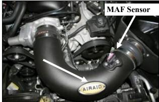
15. Install the Airaid Intake Tube into the hump hose first, and then into the reducing coupler. Adjust for fit, and tighten all four hose clamps. Next install the MAF sensor into the tube and secure it using two 8-32 x 3/8" button head screws. Apply the Airaid Decal onto the Intake Tube a shown.
