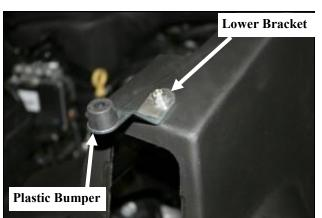
9. Turn the CAB upside down and mount the lower bracket to the bottom of the CAB using one 1/4-20x3/4" hex bolt, 1/4" flat washer, and 1/4" Nylock nut as shown. Next using one 8-32x5/8" button head screw, and one #8 Kep nut, attach the plastic bumper to the bracket as shown.
