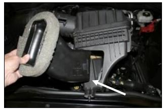
**6.** Squeeze the sides of the factory intake scoop and remove it from the factory airbox. It will be reused in step
