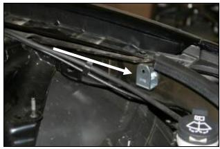
**12.** Replace the ground lug from step #11 with the ground bracket as shown using the 6mm hex bolt, and lock washer.
