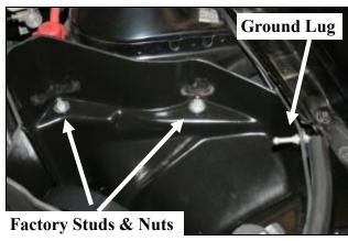
13. Install the Airaid CAB assembly into the vehicle locating the factory grommets over the factory studs. Reinstall the factory nuts from step #3 onto the studs. Reinstall the factory ground lug thru the CAB and thru the side bracket using one flat washer, and one 6mm flange nut. Refer to the line drawing on the first page for reference.
