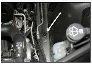
**5.** Use caution not to loose the factory grommet when you remove the air intake assembly. It will be needed if you ever want to reinstall the factory intake assembly.
