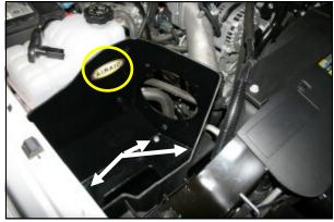
**4.** Install the Airaid Cool Air Box (CAB) (#3) into the vehicle as shown, replacing the factory air filter. Install three M6-1 x 25mm bolts (#9), and three flat washers (#7) thru the bottom of the CAB and into the factory captured nuts. Leave the bolts loose for now. Apply the Airaid decal inside the Airbox as shown.
