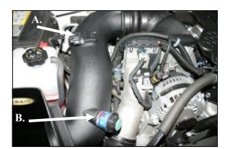
7. A.) Reinstall the Mass Air Flow sensor into the Airaid Intake Tube using two 8-32x 3/8" button head screws (#8). Do Not Use The Factory Screws!
