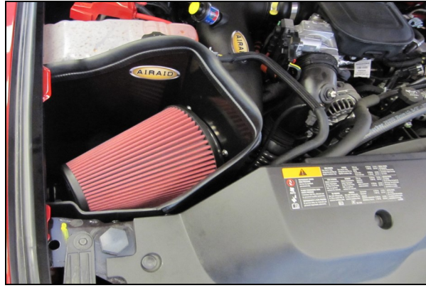
11. Install the Weather Strip (#5) onto the Airaid Cold Air Box. ( Hint: Start from one corner and work your way around for ease of install. )
